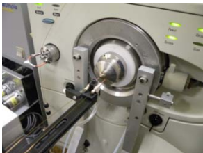
Dual Column T-Assembly for N 2 purge or sheath gas options
