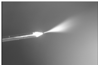
Nano-LC column with fritted, tapered end. The column exit is the spray emitter.
