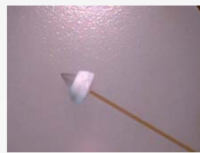
A nanoLC packed column inserted into a punched-out nozzle
