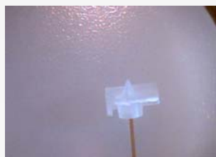
A nanoLC packed column inserted into a sliced nozzle
