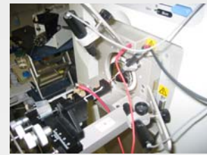
The nanoLC column with integrated nozzle was held with a holder which was in turn placed on the nanospray interface of the MS. HV was supplied through a T junction.
