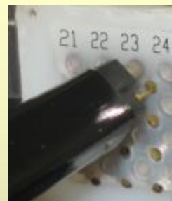
Four chips are tiled into a 16-nozzle configuration. The reservoirs in the back of the plate are sealed with a silicone sealing mat with slits that are reclosable.
