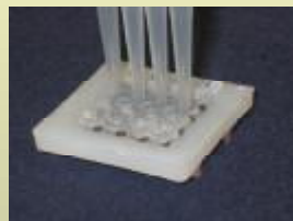
Samples are preloaded into the reservoirs with pipettes through the openings in the reclosable mat.
